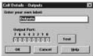
Fig 2.1. Outputs command Cell Details box for a 16F84 chip (eight outputs).
